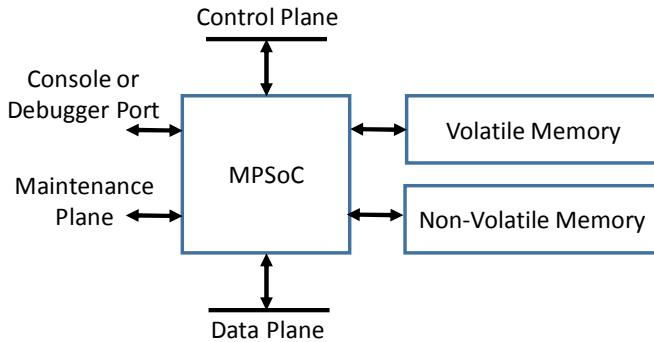
Figure 1: Common processing/memory node for a SAN architecture
